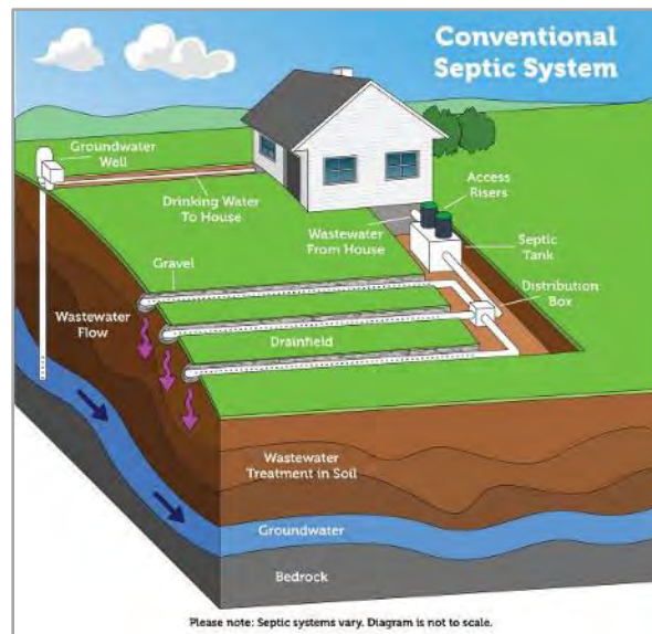
Figure 5.4 Diagram of a conventional septic system. Source: U.S. Environmental Protection Agency (USEPA)
